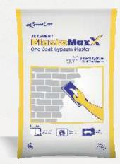
JK Cement PlastoMaxX is a gypsum based one coat plaster suitable for application on brick, block and concrete surfaces. Its vermiculite based β-hemihydrate formulation ensures working and setting characteristics. Its lightweight aggregates improve the plaster workability, coverage, application and post usage behaviour. It provides a smooth matte finish to the surface and makes it ready for painting.
